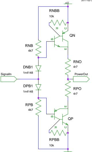
Sziklai output boosters are nearly identical to Darlington, so only part is shown. The only real difference is the "stacked" transistors, the ordering, and the base to emitter resistors. Sziklai is often popular because the extra bias diodes are not needed.
