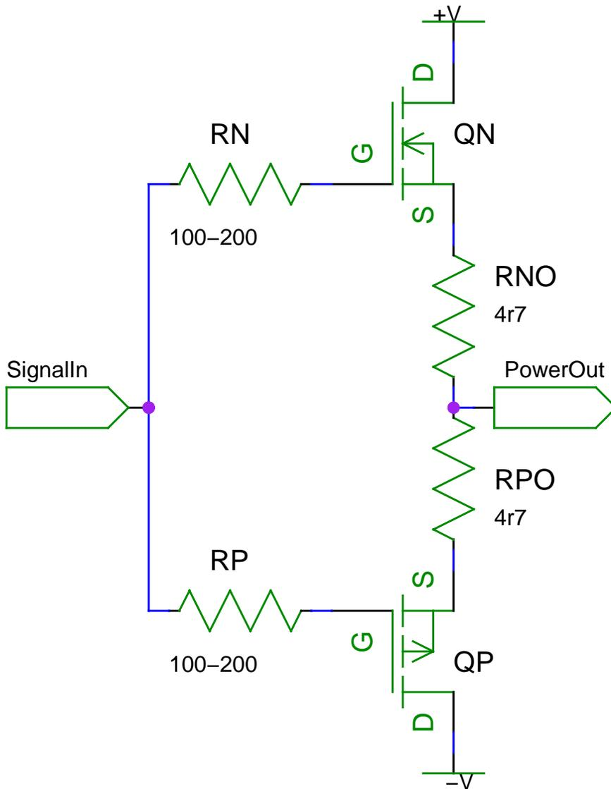
MOSFET output boosters are nearly identical to BJT, so only part is shown.
