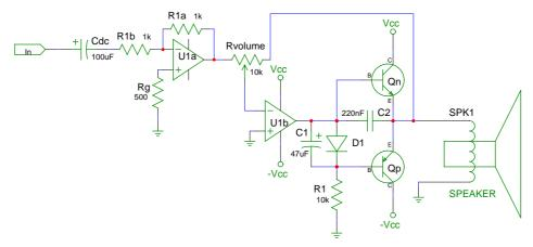
This is a Class B audio amplifier with minimal crossover distortion. Build one amplifier for each channel (2 total for stereo). Boosters like this need exceptionally clean power rails to minimize noise.
