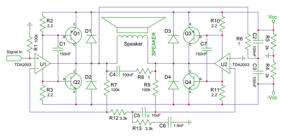
200 Watt Bridged Amplifier, 4-16ohm Speaker, 24-36v Power Rails, 5A.
