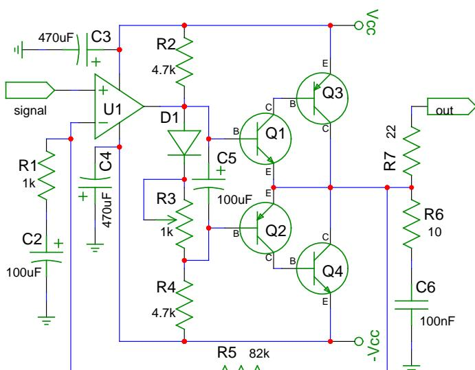
18 Watt Audio Amplifier (+/-22v Rails, Drives an 8ohm Speaker, 30-20kHz -1db)
