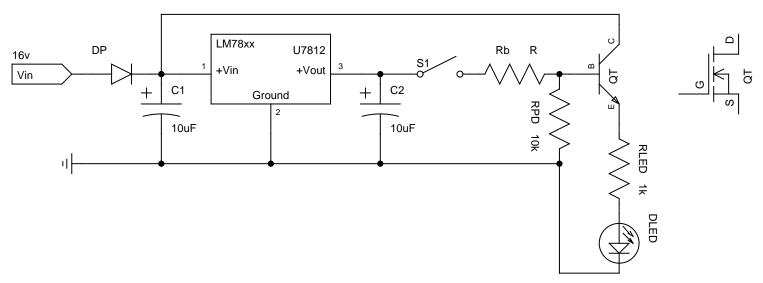
Plug in the transistor in question (NPN or N–MOSFET) where the transistor is shown.
