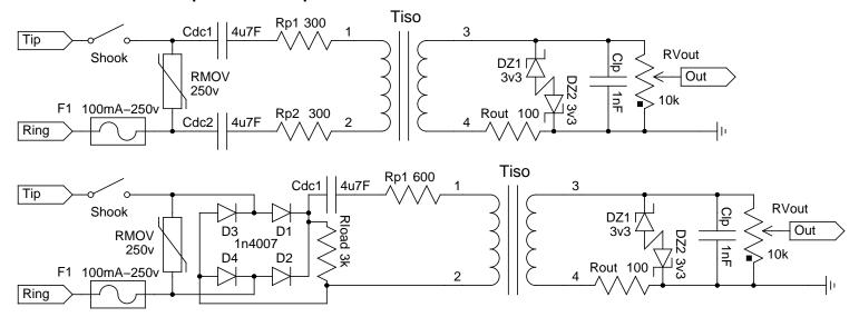
This is a circuit for a land line telephone tap directly from the wall outlet suitable for a recorder. The design goals are a clean audio signal and minimal phone line load/impact.
