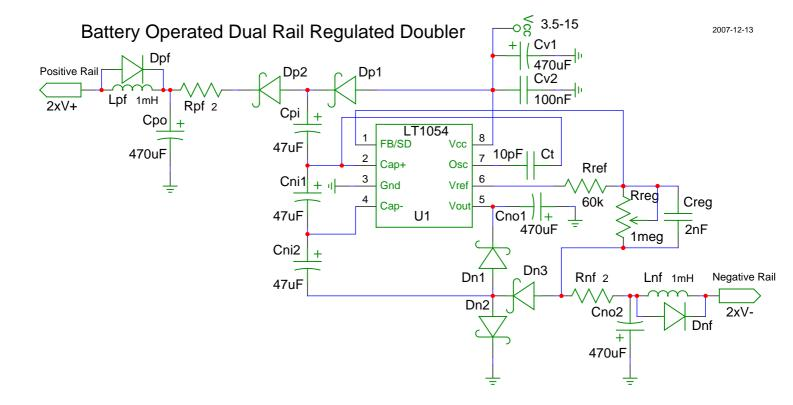
This circuit is for a regulated dual rail power supply operated from a wide battery range.
