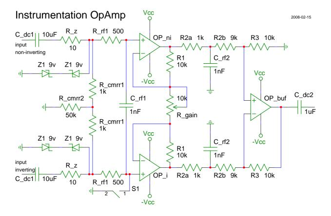
The 2 input buffers (OP\_ni and OP\_i) allow for simple gain and impedance matching to the differential amp. If the impedance is imbalanced, CMRR will be much lower. Properly balanced, CMRR can be over 50db. If R1=R2=R3: gain = 1 + 2R/R\_gain. If R's are not equal: Vo/Vs = (1 + 2 \* R1/R\_gain) \* (R3/R2).
