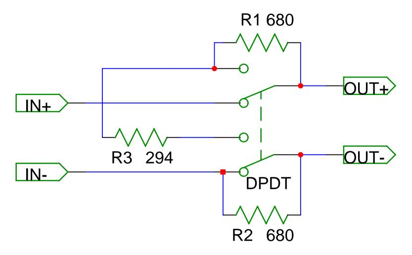
Flip DPDT switch for ~10db cut. Measure R1 and R2 to be as close as possible.
